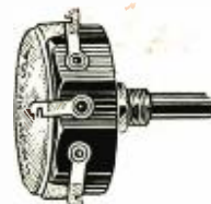
"PS8" Control Without Switch
