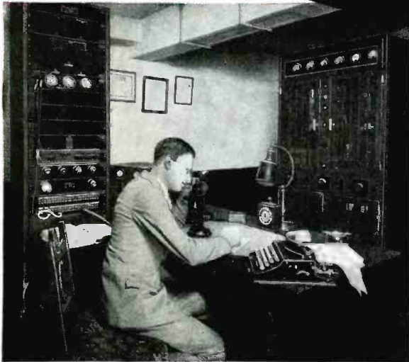
Western Electric 12A Transmitter (right) and 9A Speech Input Equipment (left) as installed at Station WHAT, Philadelphia
