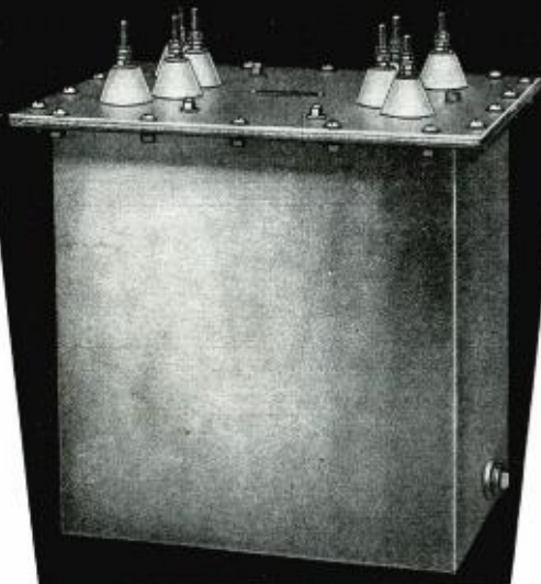
Output transformer for use between push-pull, class "B" stage using 204-type tubes and a class "C" amplifier. Operating level + 50dB; primary 1500 1500 ohms; secondary 4750 ohms; tested at 15,000 volts; oil insulated.
